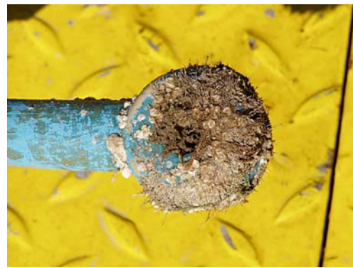
Fig. 8 Inductive-type conductivity sensor (4H Kombisonde) after 3 weeks of operation in a sensor tube (photo taken on 8 Sept 2005). The blue colour is from antifouling paint. Coating of the central bore with antifouling paint is not feasible since this would affect the form factor of the sensor and hence its calibration. The bore is therefore starting point of Barnacle and Cyclops colonisation
